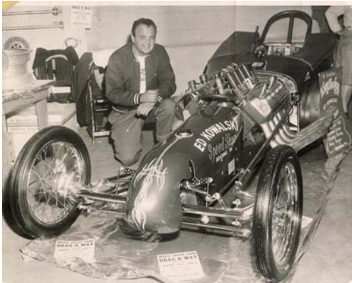
Ed Kowalski with his injected Hemi A / Fuel Modified Roadster, featuring an aluminum body by Hiram Hillegass
